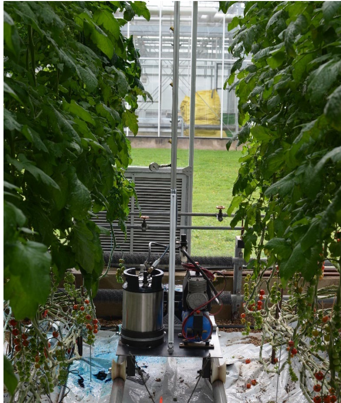
Figure 9. Vertical boom sprayer in the experimental tomato crop
